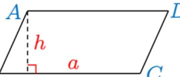
A diagram of a parallelogram with vertices labeled A, B, C, and D. The bottom side BC is labeled with the letter 'a' in red. A dashed vertical line from vertex A to side BC is labeled with the letter 'h' in red, representing the height. A small square symbol at the intersection of the dashed line and side BC indicates a right angle.
